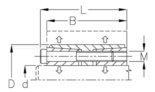
$\begin{array}{lll} \text{B mm} & = 177 \\ \text{d H8 mm} & = 320 \\ \text{D mm} & = 405 \\ \text{Fit tolerance} & = \text{Aksel h8, Nav H8} \end{array}$
